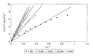
Figure 2 Stress-strain relations for NBR 40/50.
