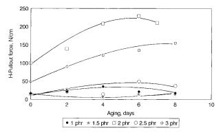
**Figure 12** Effect of aging on adhesion between NBR 34/50 and dipped nylon cords.
