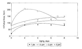
**Figure 10** Effect of aging on adhesion between NBR 40/50 and dipped nylon cords.
