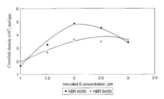
**Figure 4** Effect of non-oiled sulfur concentration on the crosslink density of the rubber mix.
