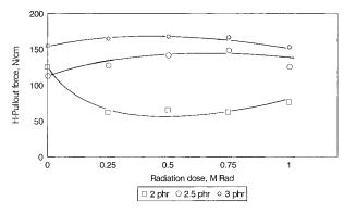
Figure 13 Effect of radiation on adhesion between NBR 40/50 and undipped nylon cords.
