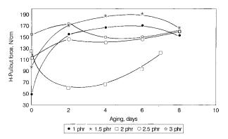
**Figure 5** Effect of aging on adhesion between NBR 40/50 and undipped nylon cords.
