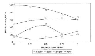
Figure 16 Effect of radiation on adhesion between NBR 34/50 and dipped nylon cords.
