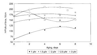
**Figure 11** Effect of aging on adhesion between NBR 34/50 and undipped nylon cords.
