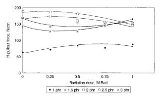
**Figure 15** Effect of radiation on adhesion between NBR 34/50 and undipped nylon cords.
