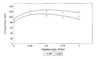
**Figure 14** Effect of radiation on adhesion between NBR 40/50 and dipped nylon cords.
