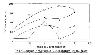
**Figure 1** Effect of non-oiled sulfur concentration on adhesion.
