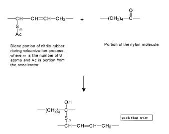
This addition reaction is believed to be enhanced thermally during aging; consequently, the adhesion strength is increased. This proposed reaction has been confirmed by reacting a sulfur containing compound like MBT, mercapto benzthiazole, and nylon by dissolving nylon cords in hot glacial acetic acid and adding MBT dissolved in dimethyl formamide (DMF) dropwise with constant stirring until addition is completed. The reaction is illustrated in the following scheme:
