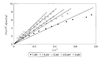
Figure 3 Stress-strain relations for NBR 34/50.
